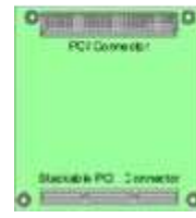
Core Module™ (104™ Form Factor) 90 x 96 mm
