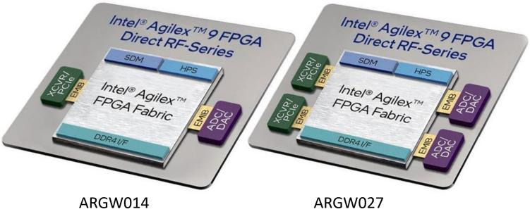
ARGW014 Intel Agilex 9 4 ADCs, 4 DACs 10 bits at 64 GSPS 1,437 logic elements 9,020 multipliers
